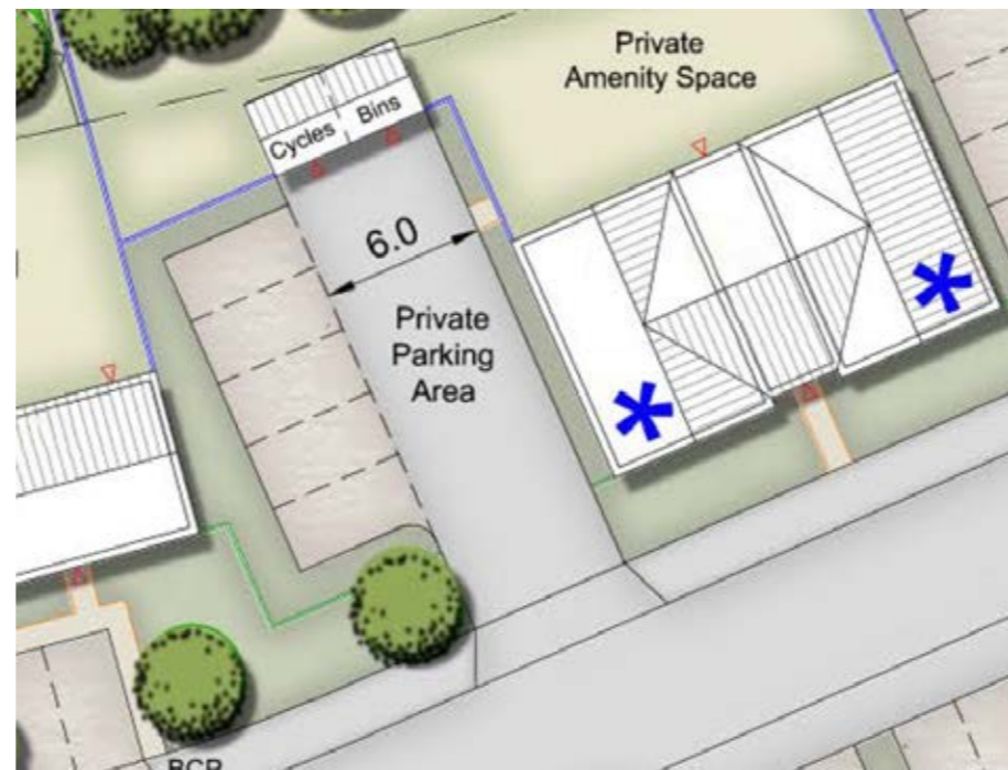
CYCLE PARKING – EXAMPLE SHOWS A SECURE COVERED CYCLE PARKING FOR A BLOCK OF FLATS, AS A COMMUNAL FACILITY.
